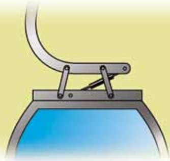
Swinging movements cushioned by hydraulic dampers
